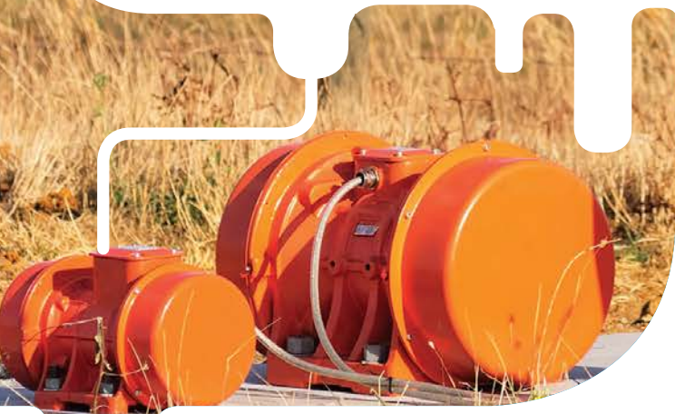
Surface orbital vibroseis (SOVs) installed and operated by Lawrence Berkley National Laboratories (LBNL)
